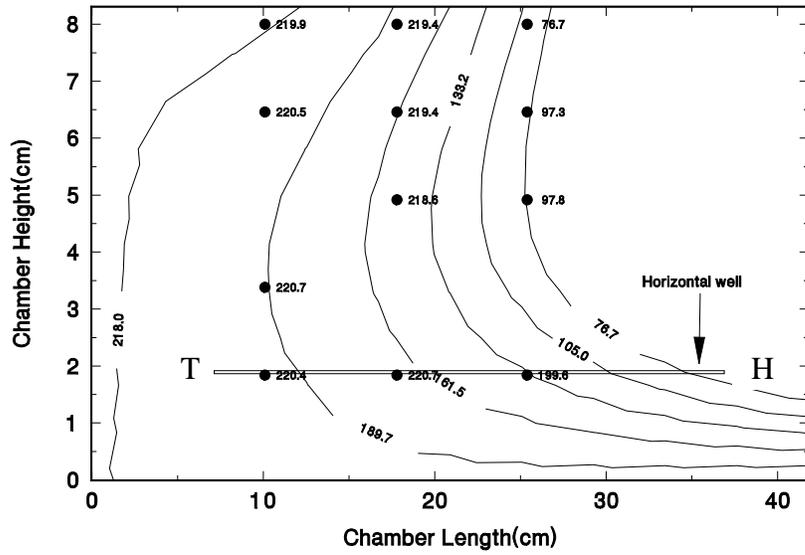
Figure 6: Test #2: TTH Steamflood isotherms in the longitudinal plane X2 at 4 hours
