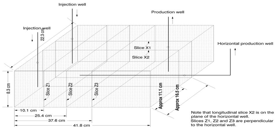
Figure 5: 3-D model -- The isotherm planes (for all tests). Well locations for tests #1 and #2
