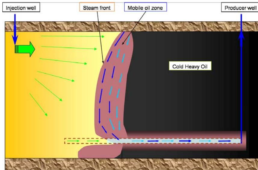
Figure 15: Schematic diagram of steamflooding in a TTH configuration; the hot oil and water are flowing down through the mobile oil zone. Some live steam is present in the horizontal section of the producer.
