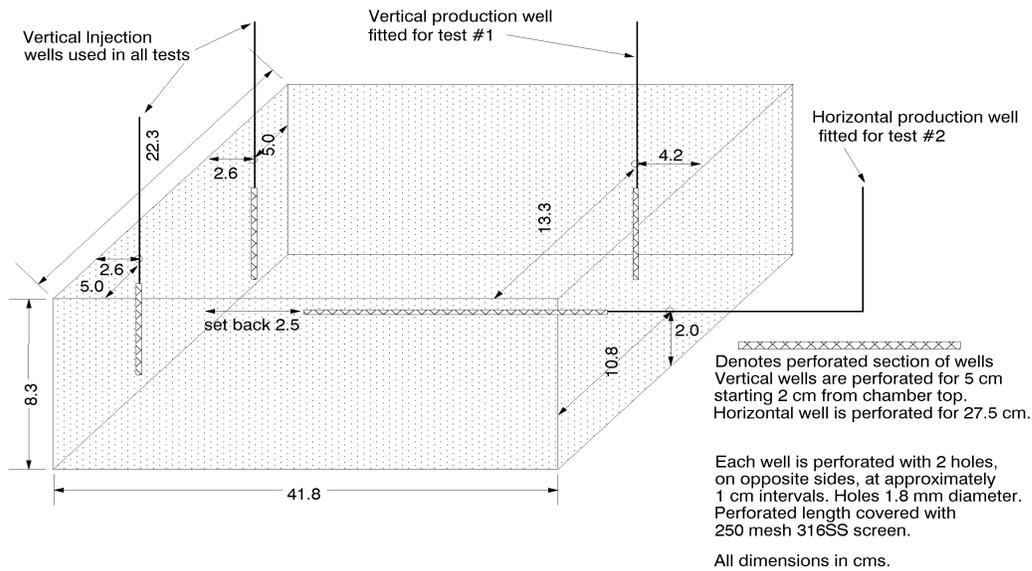
Figure 4b: 3-D model -- Cell and well dimensions for the experimental set up used in tests #1 and #2
