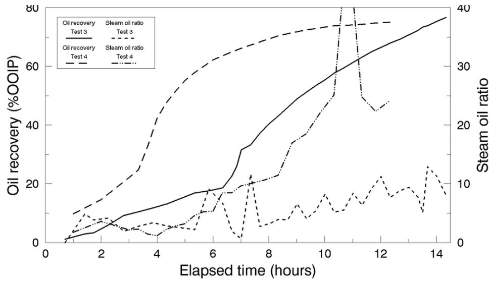
Figure 14: Comparison of cumulative oil recovered for the steamflood and thermo-solvent flood tests in a toe-to-heel configuration. (Test #3 versus Test #4) -- excluding communication phase and conventional steamflooding phase
