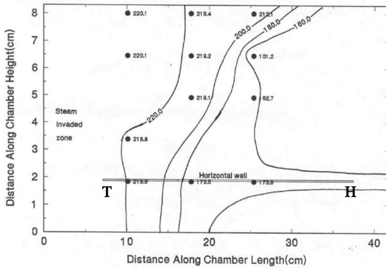
Figure 12: Test #4: Toe-To-Heel Thermo-solvent flood (TTH-TS). Isotherms in the vertical mid-plane X2 at 0.5 hours.
