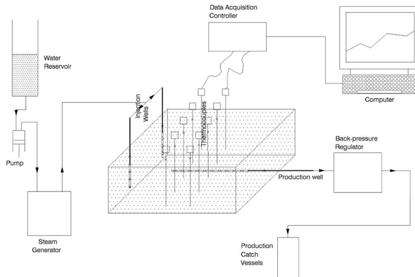
Figure 4a: Equipment schematic for the laboratory testing of steamflooding in a TTH configuration (3-D model)
