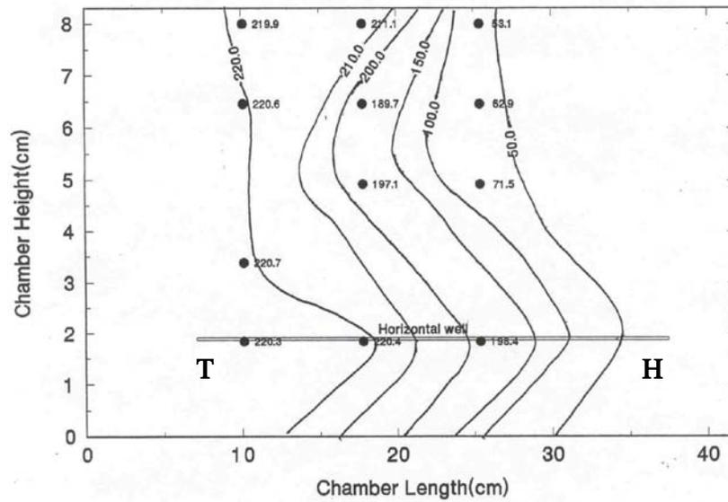
Figure 10: Test #3: Toe-To-Heel steam flood test. Isotherms in the longitudinal vertical plane X2 at 1.25 hrs.
