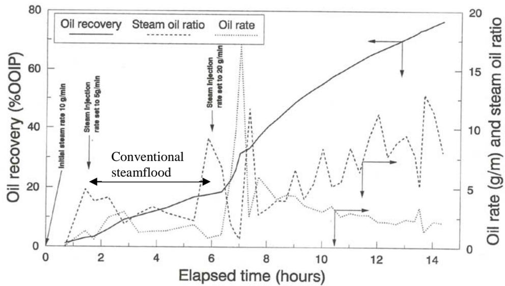
Figure 11: Test #3: Toe-To-Heel steam flood test. Variation of oil recovery, oil rate and steam-oil ratio in time
