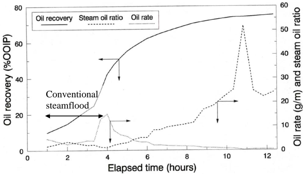
Figure 13: Test #4: Toe-To-Heel Thermo-solvent flood (TTH-TS). Variation of oil recovery, oil rate and steam-oil ratio in time
