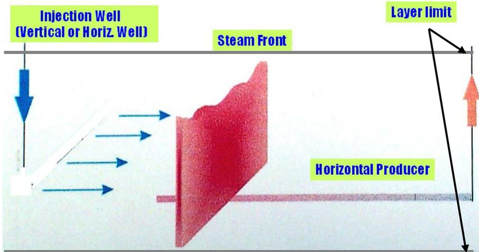
Figure 1: Concept of steamflooding in a TTH configuration
