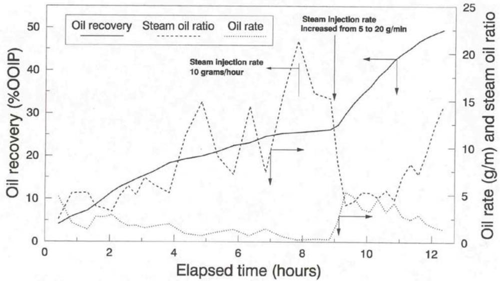
Figure 7: Test # 2: Toe-To-Heel Steam flood (TTHS) test. Variation of oil recovery, oil rate and steam-oil ratio in time
