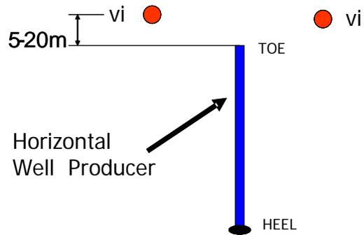
Figure 3: Bird's eye view of the THAI and TTH steamflooding processes; well configuration. Legend: VI - vertical injector
